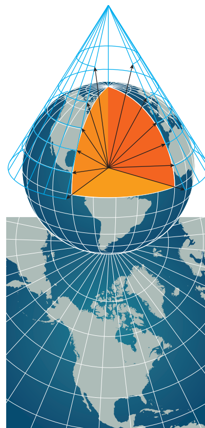
Figure 12 In a conic projection, points and lines on a globe are projected onto cone-shaped paper. There is little distortion along the line of latitude touched by the paper.
