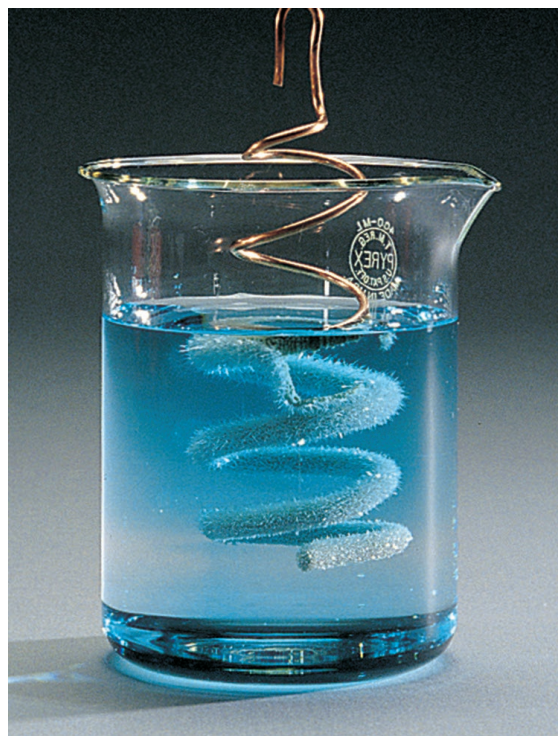
Figure 12 When a copper wire is placed in a solution of silver nitrate in the beaker, a chemical reaction occurs in which silver replaces copper in the wire, and an aqua-colored copper nitrate solution forms.
