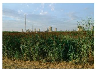
**Figure 22** Chemical waste from an industrial complex is being treated using reed beds. Bacteria and fungi in the reed beds transform a wide range of pollutants into harmless substances.
