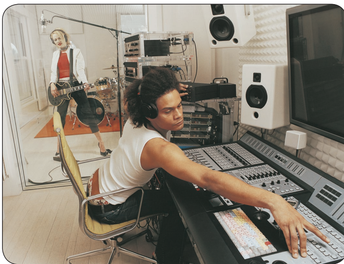
A sophisticated audio console manipulates sound electronically, making sounds sharper or fuzzier, with more echo, or more treble or bass. Its multitrack mixing and sound enhancement capabilities are most useful during postproduction.
