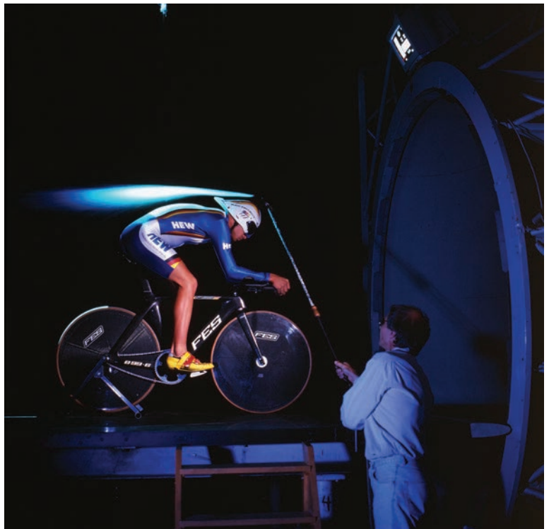
AN AERODYNAMICS EXPERT LOGS RESULTS FROM A WIND TUNNEL TEST FOR CYCLING CLOTHING AND RACING BICYCLE DESIGN.
